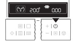
3. Using the + or - button, set the desired cooking time.
